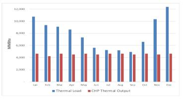
Option 2: System based on the minimum addressable thermal (1.7 MW CHP)
